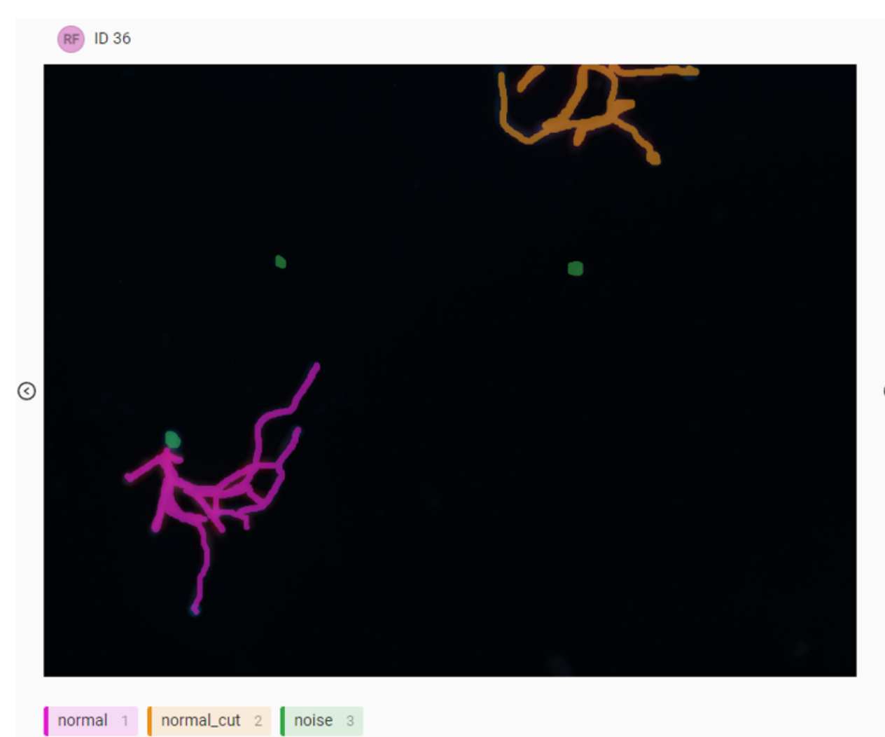
Fig. 3. An example of labelling an CWT image with the Label Studio Program. In addition to labelling living and dead plants, we generated tags to identify instrument-generated noise and plants cut during the image patch extraction process. Although not initially used, this information holds value in enhancing the system's effectiveness.
